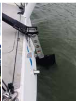
Carl Crafoord fitted a temporary rudder to get the boat home.
