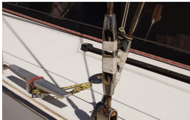
Using the KISS principle, Great White simply tapes up the offending cotter pins.
