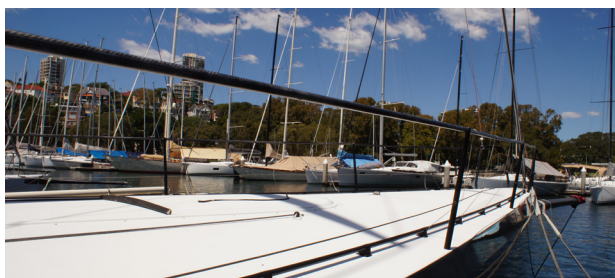
While the black carbon fibre may look sexy, we all don't have to be like Ichi Ban. You can cheaply replace this with plumber's plastic pipe.
