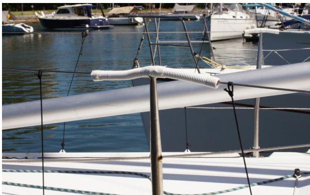
Inexpensive to buy, simple to install and easy to replace, these stanchion guards do the trick on Next.
