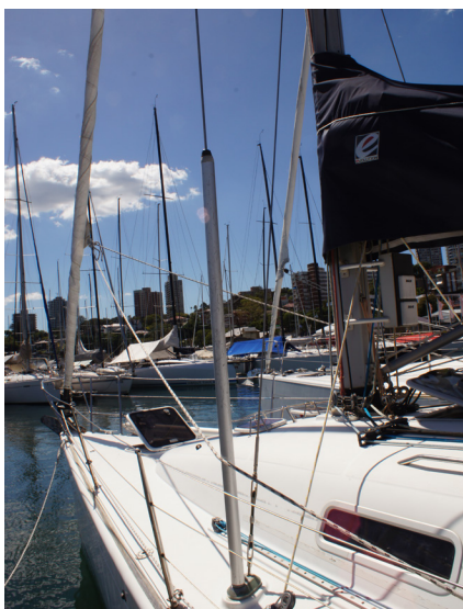
The height of the plumber's pipe on Blue Moon helps the headsail bend around the corner.
