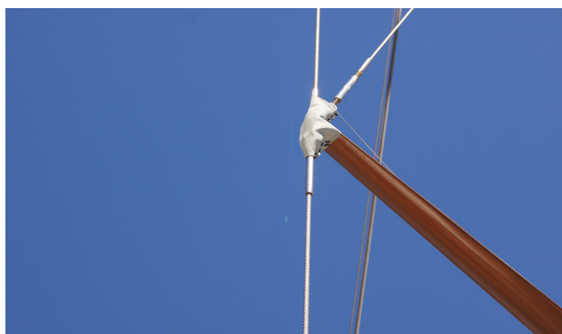
Emily is a picture sitting at the start of Arm D. Here can be seen her bespoke leather spreader protection patches.
