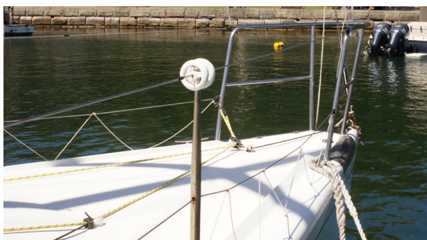
These spinning discs, seen here on Ellipse, not only protect the headsail from the stanchion, but also assist the sail in flipping over the lifelines.
