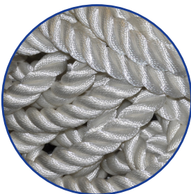
This picture shows modern nylon rope, hawser laid.
