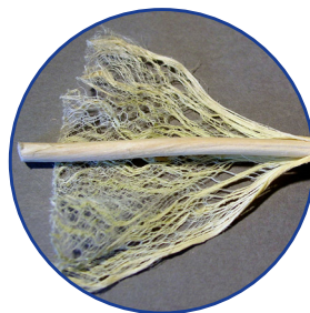
This picture shows the way the fibres are stripped from the stem of the plant.
